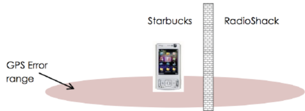
Fig. 4. Dividing wall problem [18]
